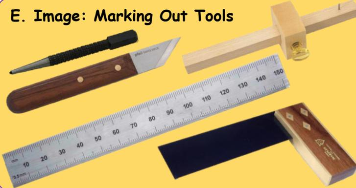
**C. Key Knowledge 2:** Consider joining two more complex shapes together temporarily with double sided tape to allow you to cut once and produce two pieces identically and accurately with less effort and saving time. Hold the **Try-Square** flat against a straight edge to allow you to draw a 90 degree line accurately. Always measure using mm as they are more precise than cm. This will allow for more accuracy and perfect sizes.
